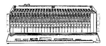
The modular RAC chassis mounts in a standard relay rack within the central office/central exchange and transports HDSL traffic to the CO's Ethernet network or the local backbone. With a 10Base-T Ethernet interface, the LAN module provides connectivity to a LAN switch or router. The RAC is fully NEBS compliant and fits into a central office 12" deep footprint.
